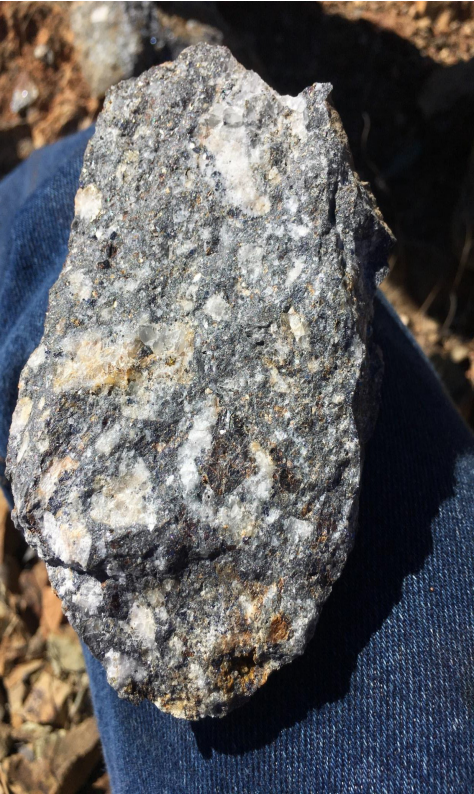
Brecciated quartz vein cemented with sulfides (sphalerite, galena)
