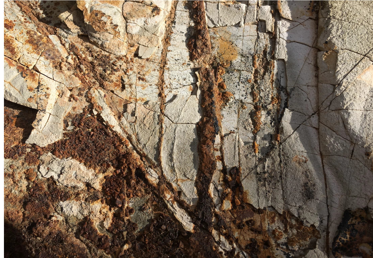
Micro veinlets of goetite and limonite in agilized sediments.
